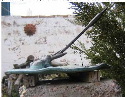
wedge may be used to tilt the entire dial such that the final style is tilted at your latitude. Living at latitude 32 degrees, I needed a wedge of 14 degrees.
