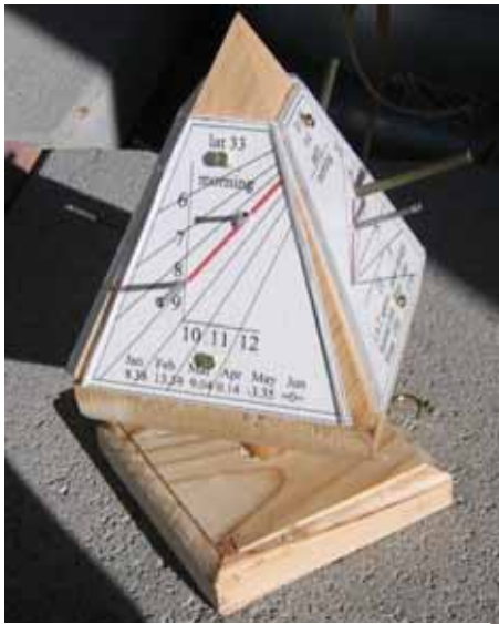
The completed dial, showing 7 am on the southeast and north east faces.
