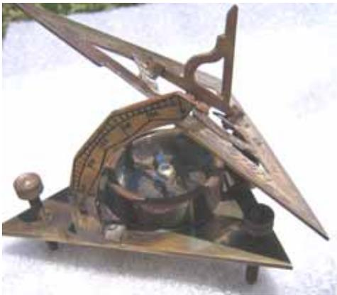
At latitude 8 on the protractor scale the gnomon's style is set to 90 degrees.
