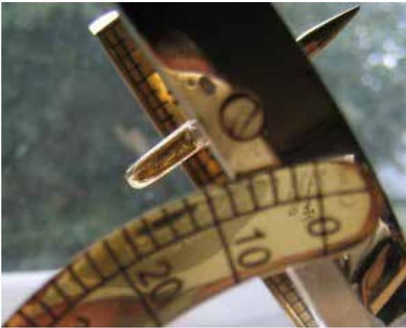
This dial was set to latitude 35 approximately using a construction protractor. The latitude guide has two problems. First it shows about 8 to 10 degrees, secondly the line of the armillary dial plate isn't even parallel to the lines on the protractor of the dial
