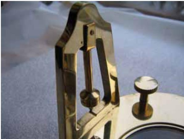
This dial comes with a level, it is a plumb line and it can only move in one axis. A dial plate when leveled should be level in all axes, which is why the plumb line should be a thread, or two spirit levels used.
