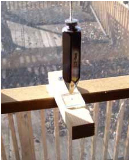
A small piece of wood was placed on the cross piece, and a reflective surface added. Again, it was leveled in all axes.
