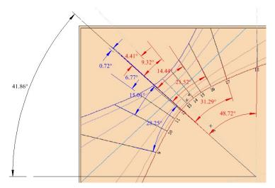
The angles can be checked by using the spreadsheet, as before, except that the base time would need to be adjusted by the longitudinal difference, being 1° for 4 minutes. In this case, the SHADOWS software was used and the angles found to be in close agreement. Since the geometric method uses the local solar noon as the base, and SHADOWS does not, it is important to add into the SHADOWS depiction the local solar noon, and measure angles from thence.
