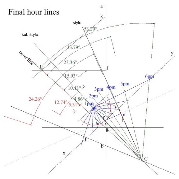
Finally the hour line angles are measured, for consistency they were measured from noon. Of course the angle of the noon line with the horizontal or vertical was previously determined on the first of the geometric worksheets.
