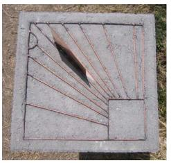
Every hour the shadows were checked on the cardboard dial plate, with consideration to the equation of time. If for example the EOT table said 10 minutes was to be added to sun time, then on the hour it would actually be 10 minutes past, so the dial would be checked 10 minutes after each hour.
