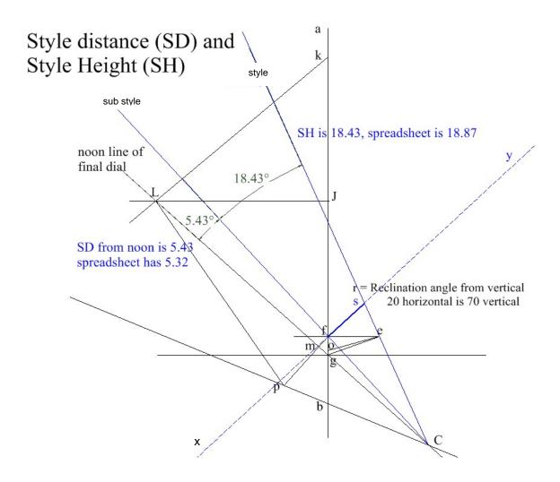
STYLE HEIGHT (SH): through point (f) draw a line (xy) which is perpendicular to the recently drawn sub-style.
