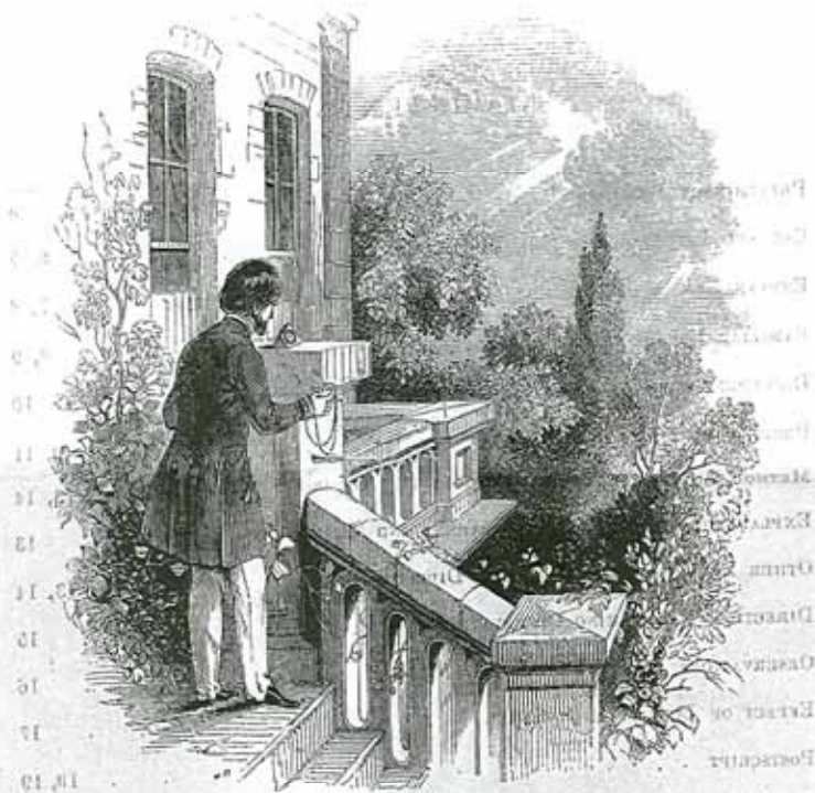
ILLUSTRATION OF THE SIMPLE MODE OF TAKING AN OBSERVATION WITH THE DIPLEIDOSCOPE.
