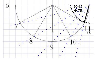
This is explained simply since each is an isosoles triangle. Since an angle at the base is 75 degrees, being 90 degrees minus the 15, and since the other base angle must be the same as both are on the circumference, and both go to the semi-circle's center, then they total 150 degrees, leaving 30 when subtracted from 180. Thus, 30 degree radials from the dial center are drawn, which can easily be translated into linear distances once the radius of the semicircle is known.
