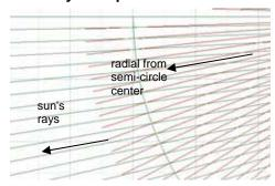
To the left are shown 1 degree lines from the opposite style which is to the right, and 2 degree lines from the semi-circle center which is from the top. The sun's lines intersect perfectly, they are close to perpendicular with the dial plate, so accuracy is highest.
