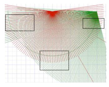
On the left the complete picture of 1 degree solar rays and their intersection with the 2 degree radials from the semicircles center can be seen, and the three boxes correspond to the three expanded pictures above.
