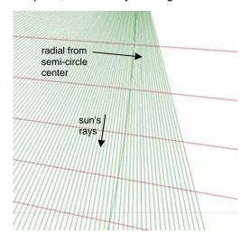
To the left are shown 1 degree lines from the style which is to the top right, and 2 degree lines from the semi-circle center which is from the top left. The sun's lines intersect perfectly, they are close to flat with the dial plate, so accuracy is lowest.
