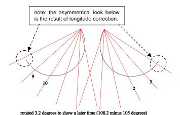
To the left, the radials have been rotated 3.2 degrees, being the dial location (108.2) minus the legal meridian longitude (105). This is how longitude correction is applied to a dial when the basis for the dial design is the 15 degrees per hour radials. Except for armillary and equatorial dials, moving a dial plate relative to the stylus does not retain relative angles thus as a rule it is an incorrect method of adjusting a dial.
