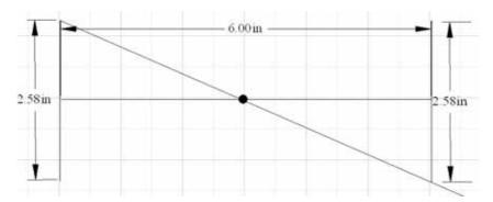
In this case, we can halve the length of the style, and thus dial plate. Thus a six inch diameter semi-circle need only have a width of 2.58 inches, or in more general terms, the width of the dial plate, summer to winter, is 2.58/6 inches or 0.48 times the diameter. Or in very loose terms, the dial plate is about as wide as its radius.
