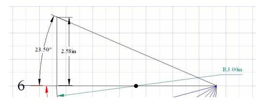
However, this assumes a nodus is used. It must be remembered that the gnomon-less dial has two styles, and if declination lines or calendar lines will not be used, then all that is needed is to ensure that the style's shadow is always on the dial plate. So the southernmost tip of the style can be used for the winter shadow, and the northernmost tip for the summer shadow.
