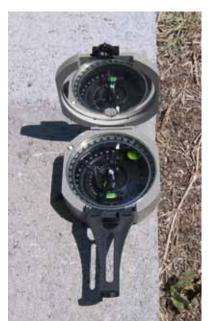
Then the gnomon track was laid out, and this used a Brunton compass for alignment. The magnetic
