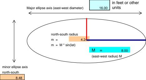
The ellipse is not drawn to scale, the pictorial is simply to help orient the diallist. At this point an ellipse can be drawn and the angles from the ellipse center used to identify the hour points. Alternatively the east west and the north south coordinates of the points can be used to locate the hour points.
