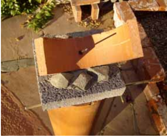
The dial plate tacked to a base and to some small rocks, using Versabond.
