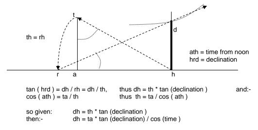
The distance up the hour line for the point on which the declination (calendar) line will lie is equal to the style linear height times the tangent of the declination all divided by the cosine of the time. This is repeated for several of the hour lines, then the points joined to form a hyperbolic curve for the solstices, or a straight line for the equinox.
