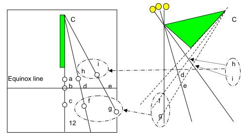
When this process is completed for as many hour lines as desired, the dots are connected and then the declination lines drawn.
