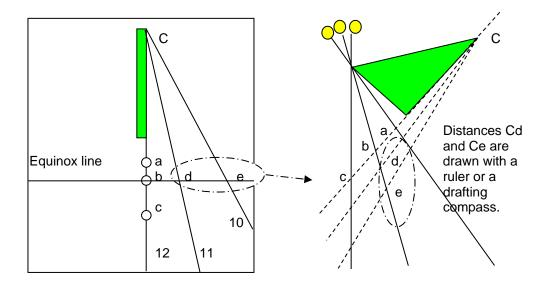
The equinox line is then drawn perpendicular to the noon line, and it produces equinox intercepts for those additional hour lines, d and e. Distances Cd and Ce are then located from the left dial plate to the right hand picture on its equinox line. This produces two more hour lines on the right hand side picture, Cd and Ce. Those hour lines on the right hand side do not have angles that match their hour lines on the dial plate, and this is because this is a projection.
