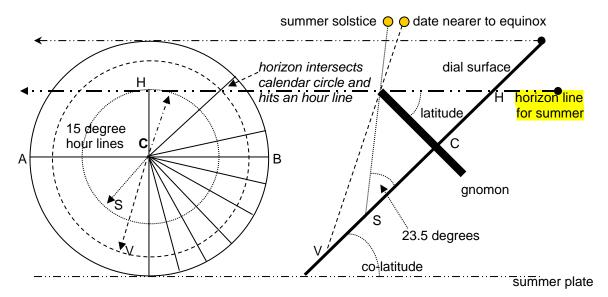
A horizon line is drawn from the nodus as shown above, and it crosses the 15 degree hour lines and the declination circles. For any date, the declination circle is found, and sunrise or set is the intersection of that declination circle with the hour line. Winter would use the lower nodus.
