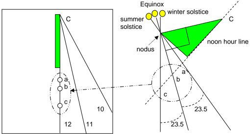
First, draw a gnomon for the dial center "C". From the nodus draw the equinox line (90 degrees to the style), and from that the solstice lines (approx 23.5 degrees on either side). The three lines (equinox and the solstices) intersect the gnomon's base line extended, or the noon line, at points a, b, and c. These three points whose distances from the dial center are Ca, Cb, and Cc are then transcribed to the dial plate (right pictorial to left pictorial).
